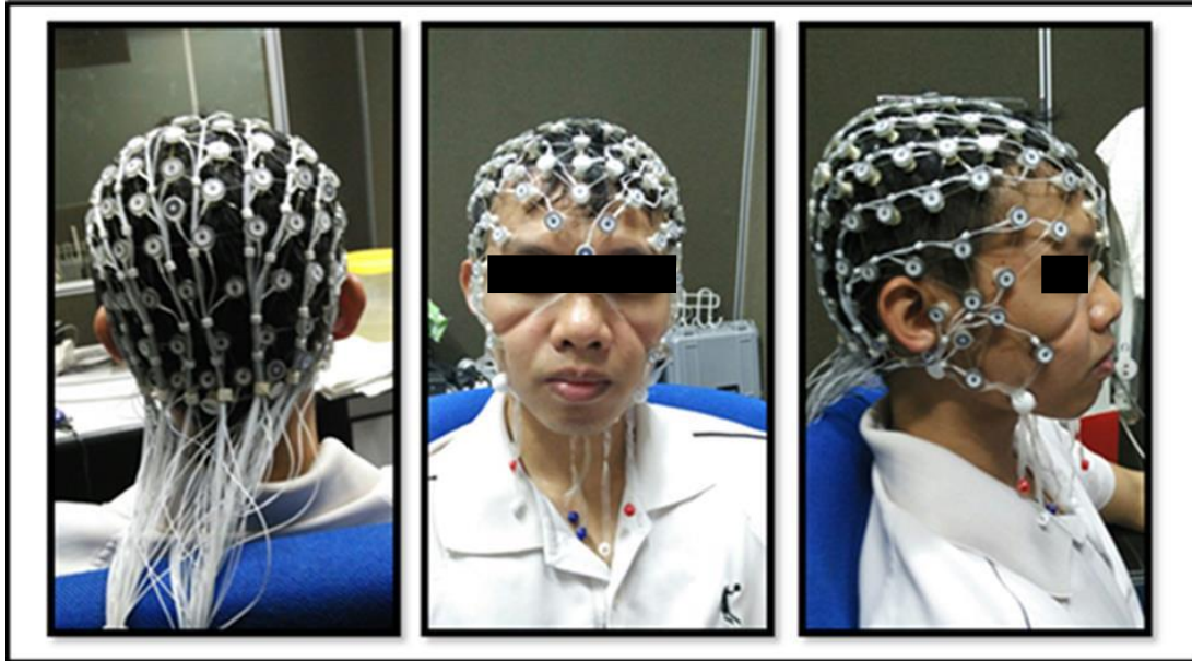
Figure 2: The 128 Channel Hydrocell GSN Layout Applied On Subject's Head
